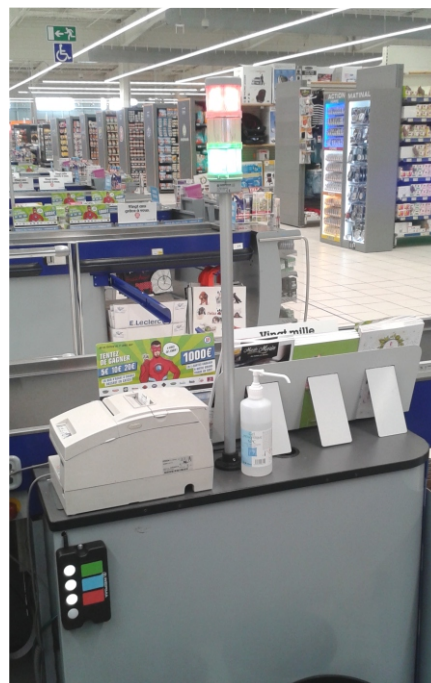
The cashier can change the lights or call for help using the Andon SmartBOX without leaving the workstation.
